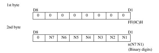
When the number of lines to be fed ( $2^{nd}$  byte) is written-in following the paper feed command ( $1^{st}$  byte), the paper will be fed by the number of lines specified. The number of lines to be fed can be specified from n=1 to 127. If "0" is specified, paper feed will not be carried out. When there is data in the print buffer at the time this command is applied, this data will first to printed out and then line feeding of "n" – lines will be performed.
